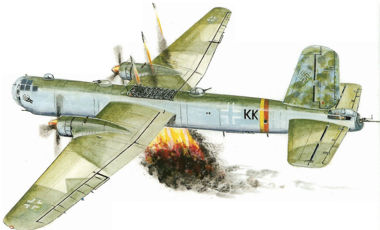
A Heinkel He 177 firing a battery of Wfr.Gr. 42 projectiles from its oblique upward-firing fuselage array.
