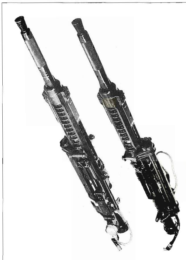
The 20mm MG FF/M with electro-pneumatic triggering. Its rate of fire was 540 rounds per minute.
