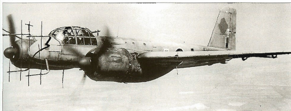
Junkers Ju 88C-6 with FuG 220 SN-2 nose radar antenna array.
