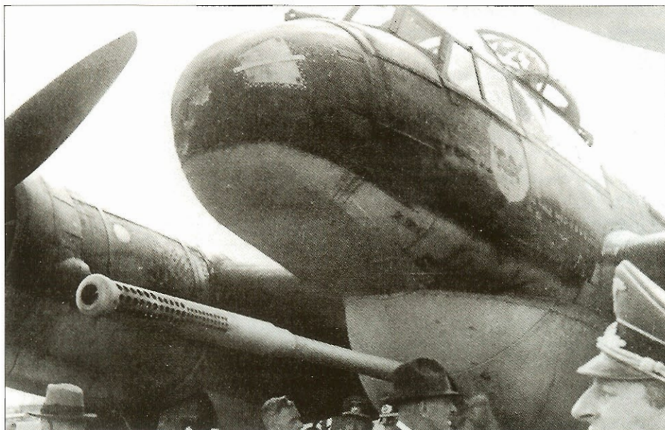
The Ju 88P-1. The BK7.5 multi-orifice muzzle brake is clearly visible.
