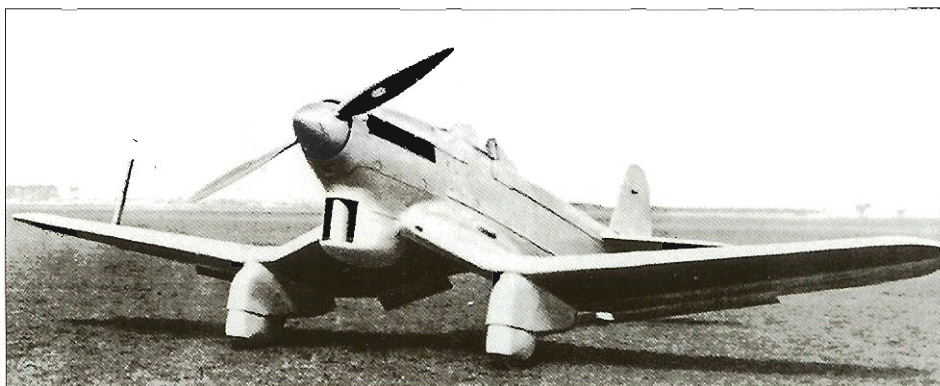
HFB Ha 137 V1 with 640hp Rolls-Royce Kestrel V in-line engine.
