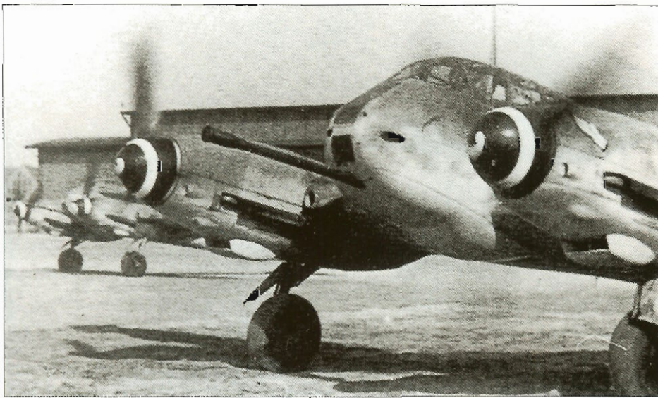
The BK 5 Bordkanone installed in a Me 410A-2/U4.
