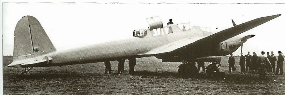
Focke-Wulf Fw 57 V1. Note that the planned 20mm cannon have not been installed in the Mauser dorsal turret.
