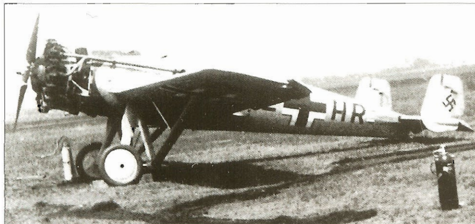
Left: The Junkers K 47 as a low-level attack training aircraft. It was used until after 1939.
