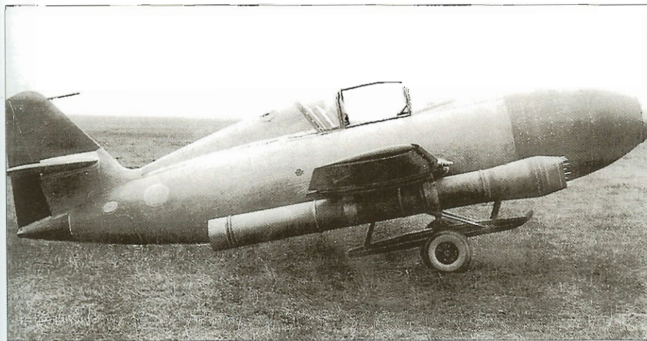
Messerschmitt Me 328 V2 with two Argus VSR 7 pulsejets.
