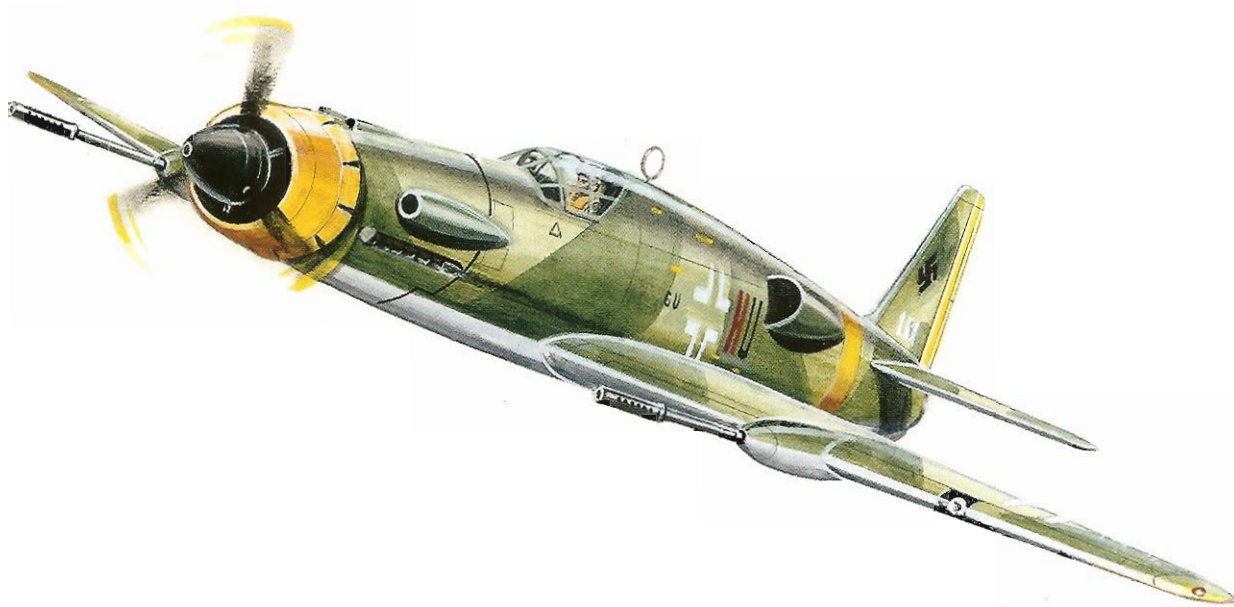
Dornier P 232/2 with fuselage lateral air intakes for the turbojet.
