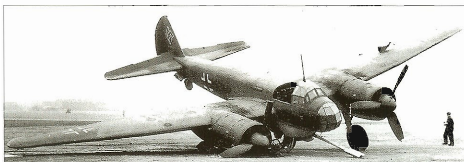
A Ju 88P-1 damaged on landing due to its nose-heavy BK7.5 cannon.
