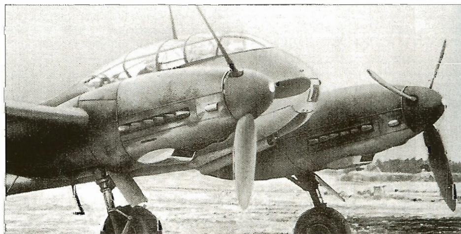
Experimental installation of a Wfr.Gr. 42 multi-round magazine as a fuselage nose weapon on a Messerschmitt Me 410A-2.
